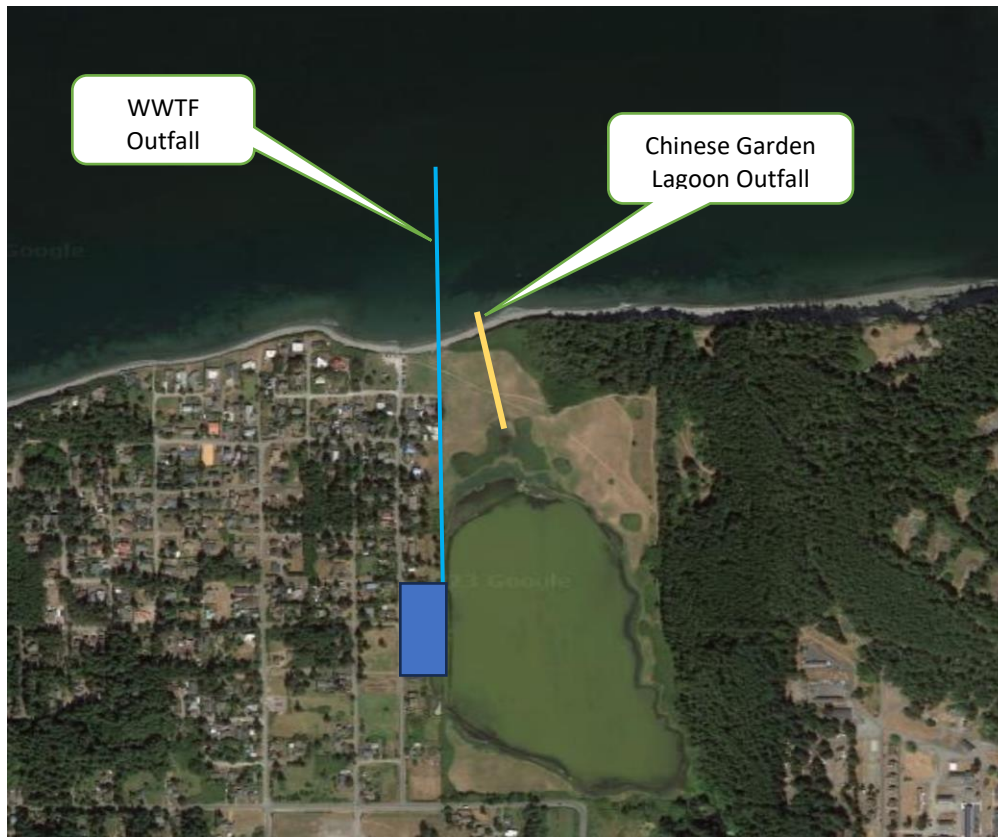
Figure 8-11 – Approximate Outfall Configuration
