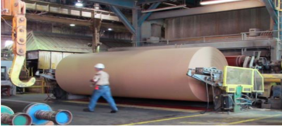
Kraft Linerboard maximum roll weight of 8,000 pounds
