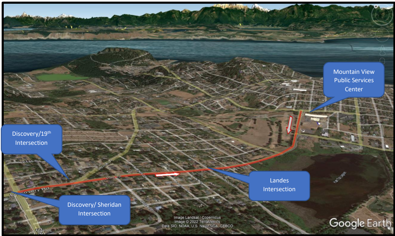
Topography Illustrating Grades on 19 th Street
