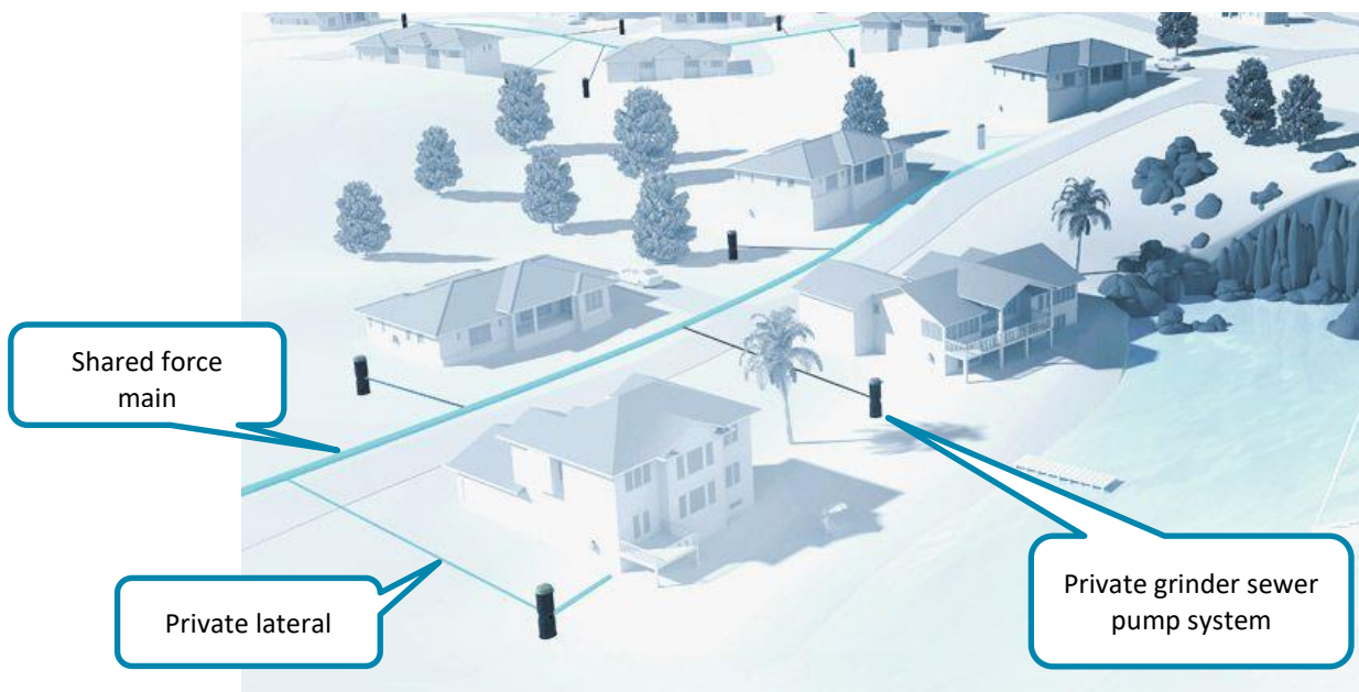
Low Pressure Sewer System Schematic. Image credit: Environmental One website.
