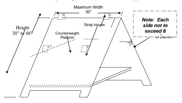
Face to be made from ½ inch exterior grade plywood. Faces are to be coupled with strap hinges. Hinges to be fastened with 1/8 inch or larger pop rivets. The heads of rivets are to be on the readable face of the sign. Use same procedure for fastening the hinges for the counter weight platform and the support.
