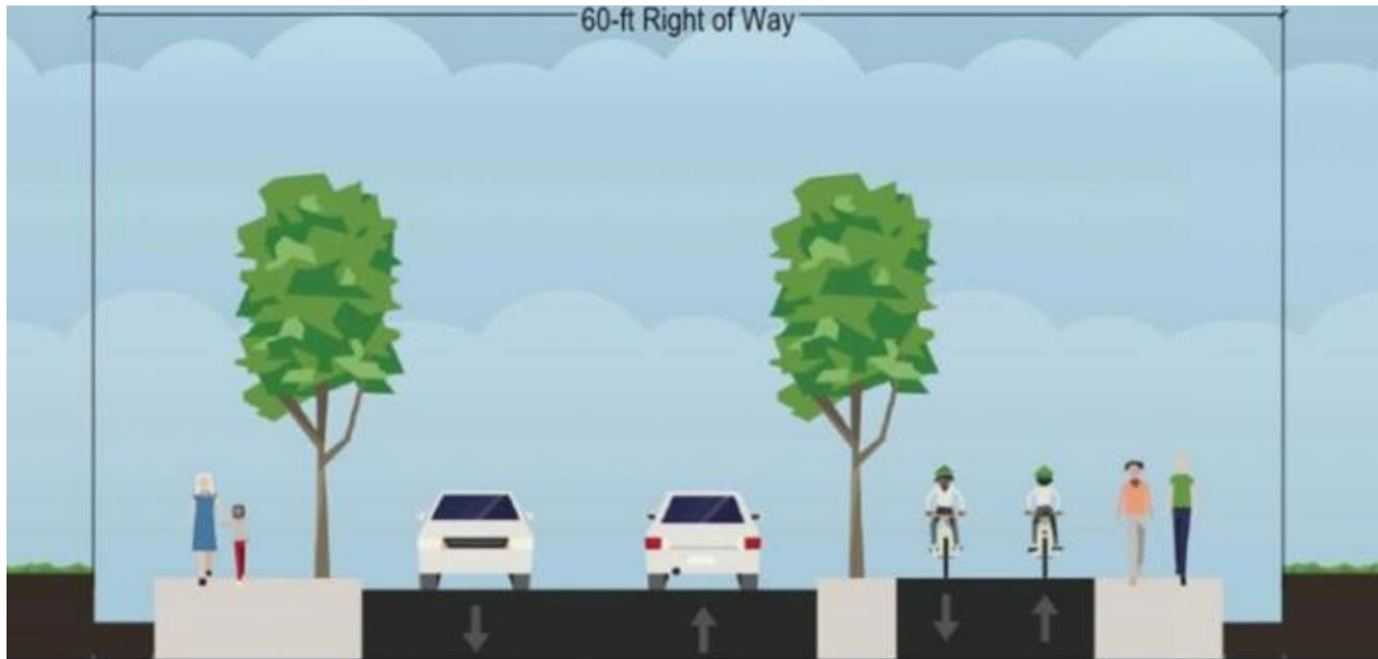
Typical Cross Section. Note the landscape strip on the left is 5-7 feet wide and will contain a drainage swale. The landscape strip on the right is 4 feet wide.
