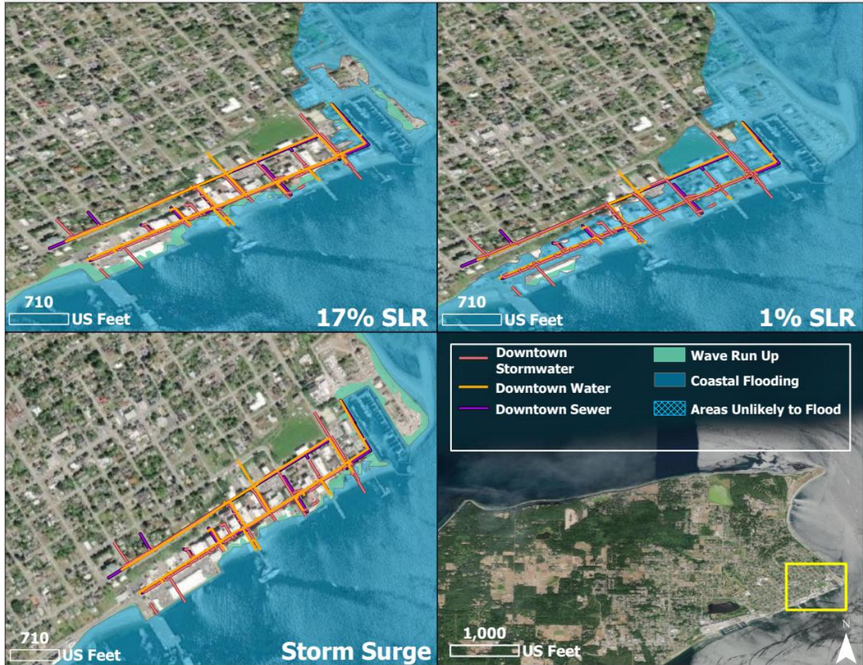
Figure 7. Downtown infrastructure exposed to different inundation scenarios. Storm water pipes are shown in pink, water systems are shown in orange, and sewer lines are shown in purple. Coastal flooding is shown in blue, wave runup in green, and areas unlikely to flood in a crosshatch blue pattern for each inundation scenario. Coastal flooding from the 17% sea level rise event and the 1% sea level rise event also take into account flooding brought on from 1% storm surge.
