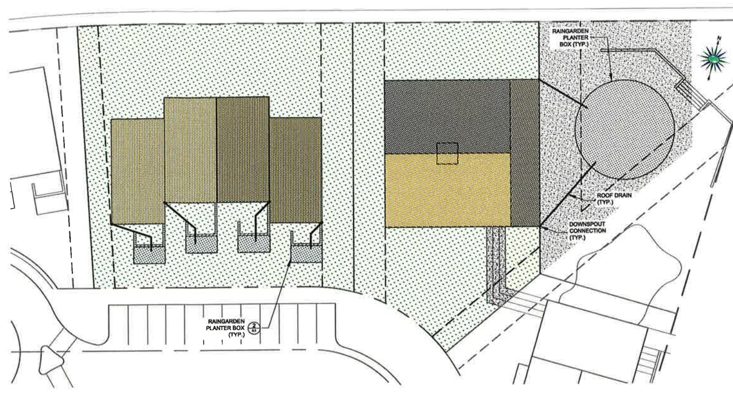
2 TYPICAL COMMERCIAL LOT STORMWATER PLAN 8.2 SCALE: 1:20
